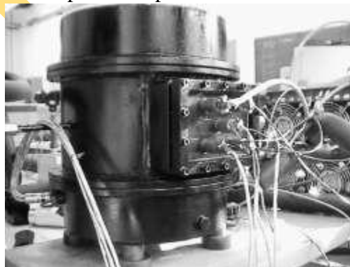
Fig5: final view of compressor with thermocouples and capillary devices
