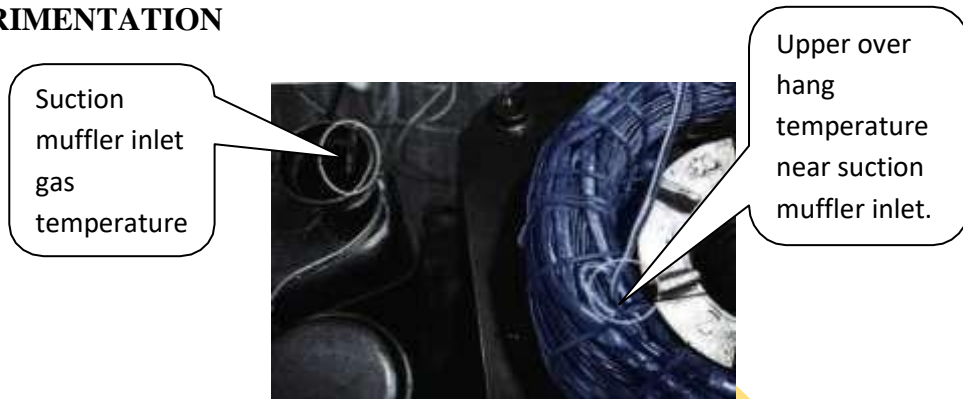
Fig:2: Upper overhang temperature near suction muffler and SMA inlet temperature
